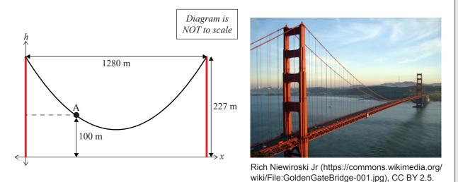
An anemometer (shown as A in the left-hand diagram above) to measure wind speed is placed on a cable at a height of 100 metres above the mean water level.
