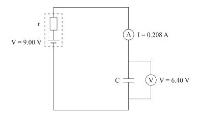
(a) At one point during the charging, the capacitor has a voltage of 6.40 V, and the current flowing in the circuit is 0.208 A.
