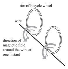
The inductive loop circuit uses Faraday's law to detect changes in the inductance when a bicycle is above the circuit. The high-frequency, alternating current induces a magnetic field in the metal bicycle rim. The magnetic field induced in the bicycle rim reduces the overall magnetic field. The inductance of the circuit is reduced, and this is detected by the traffic lights.
