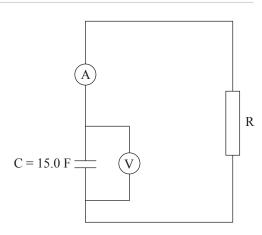
Use the graph to show that the resistor is  $4.50 \Omega$ , and calculate the maximum current in the circuit.
