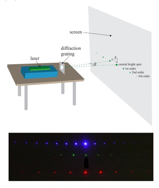
The picture above shows three different colours (from top to bottom: violet, green, and red) of laser light shone through the same diffraction grating.
